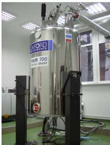
700 MHz NMR spectrometer installed in Faculty of Chemistry, University of Warsaw since 2006
