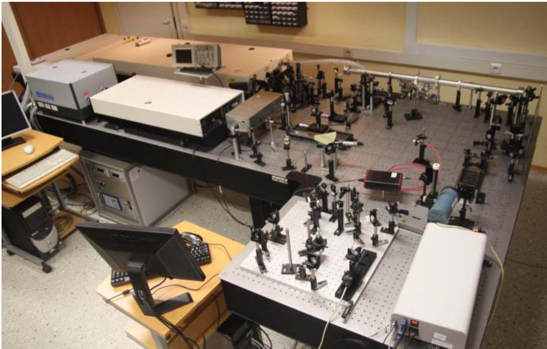
Front-end of high-power OPCPA laser system prototype located at Vilnius University Quantum Electronics Department
